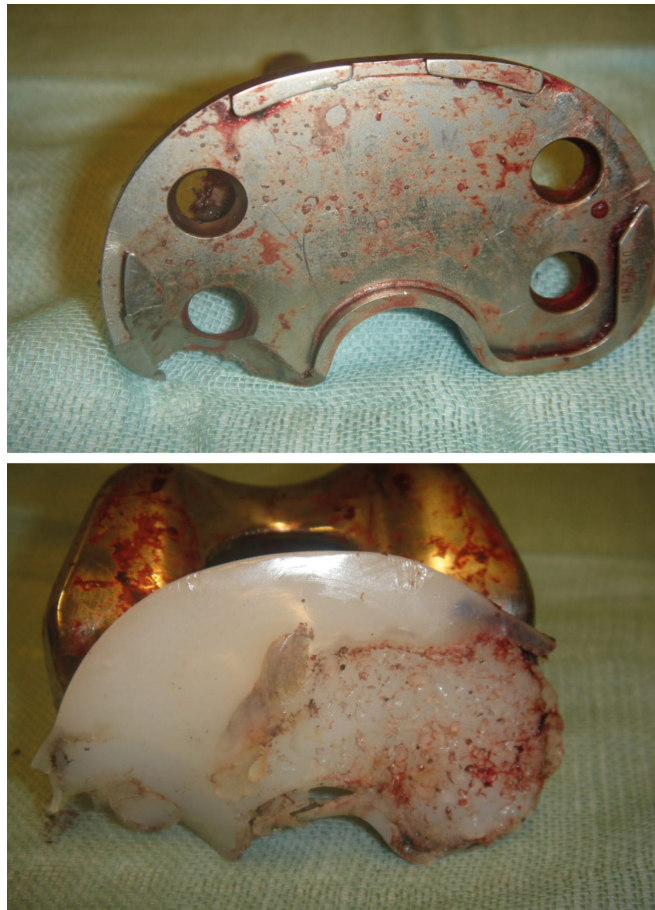
Figures 2 & 3 : Destruction of the polyethylene insert and the tibial tray observed during revision arthroplasty.
