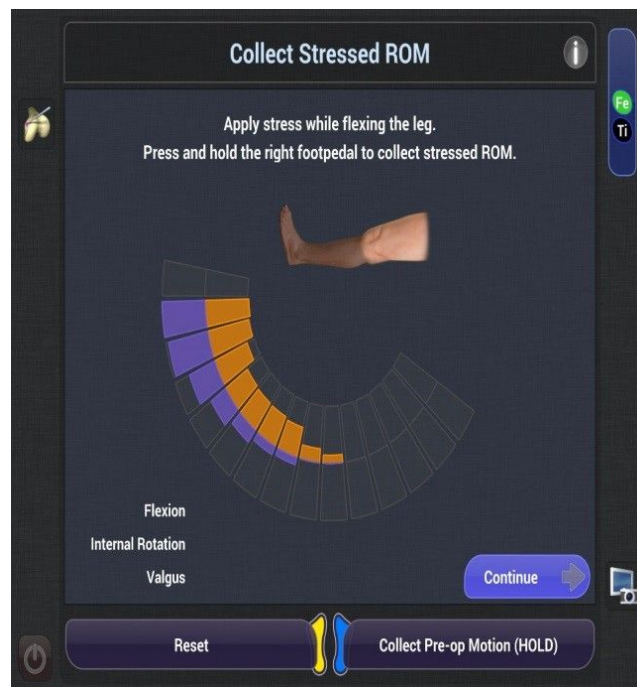
Figure 15. Collection of gap planning data prior to the procedure, across the whole range of motion
