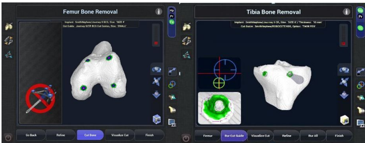
Figure 18. Placement planning for the femoral and tibial cutting guides using the robotic handpiece
