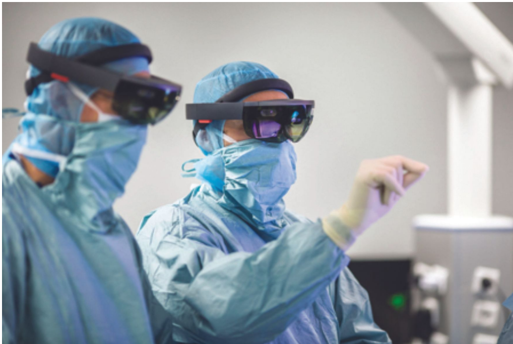
Figure 7: Using the Microsoft© mixed reality HoloLens® headset. Photo by Raphaël de Bengy. Exclusive rights: Hans Lucas. The surgeon interacts with the smartglasses by making gestures in front of the visor.
