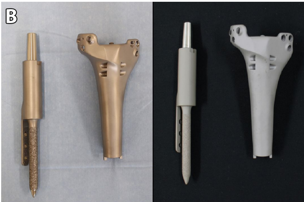
Figure 1 A to C. A. Left: 20 cm intercalary defect after tumor resection. Right: Custom-made implant with 3D printer. B. Left: Custom-made titanium implant with 3D printer. Right: The implant after surface modification with iodine (off-label). C. Left: intraoperative picture after reconstruction (off-label use), Center: Radiograph 1 year after operation. Right: Excellent bone ingrowth.
