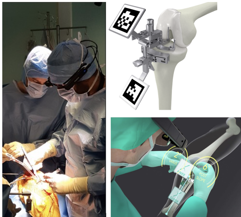
Figure 4: The Pixee Medical system is a computer-assisted orthopedic surgery solution using augmented reality to support TKA, with connected glasses and specific markers on the knee (QR-Code) providing intra-operative data on the bone cuts axis.
