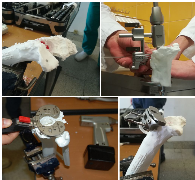
Figure 6: The 3D model produced with FDM technology and taken to the dry lab for surgical testing.
