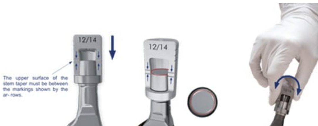
Figure 4: Compatibility test between taper of retained stem and the 12/14 adapter with BioBall® AdapterSelector® in isolated cup revision
